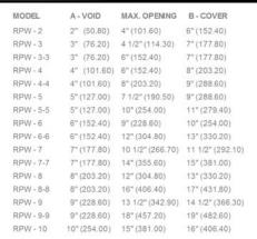
MODEL - RPW -2 ROOF PARAPET TO WALL
